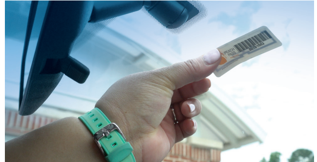
Tolls are collected electronically with a small electronic transponder.
